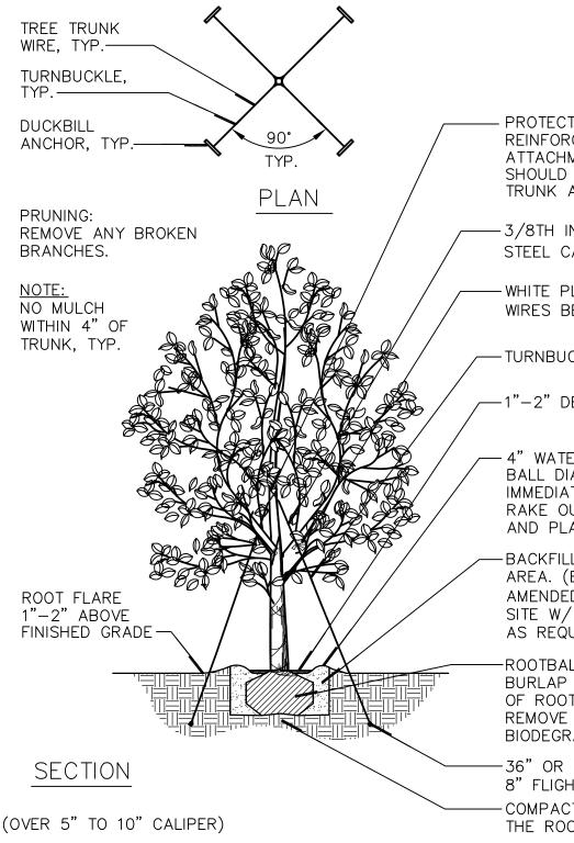
PROTECT TREE TRUNK WITH 1/2" REINFORCED RUBBER HOSE. ATTACHMENT POINT OF CABLE SHOULD BE 50-65% UP THE TRUNK AND ABOVE A MAJOR BRANCH.
